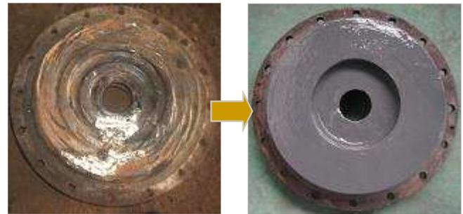
Fan pump cover's surface condition was severely damaged by corrosion attack. Successfully profiled and rebuilt by Elastomer Nusindo.
