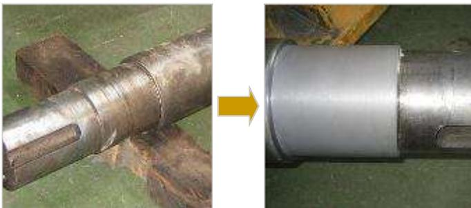
Rebuilding of worn out bearing seat on the shaft was accomplished using the Wearguard® system. Precision Finishing and Grinding was performed to achieve bearing fit tolerance
