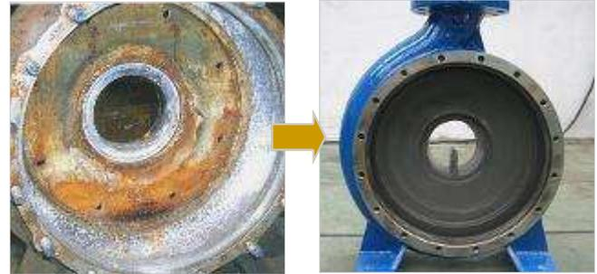
The casing of the fan pump has been damaged due to extensive wear and poor maintenance. Rebuilt to like-new condition with approximately half the cost of new one.
