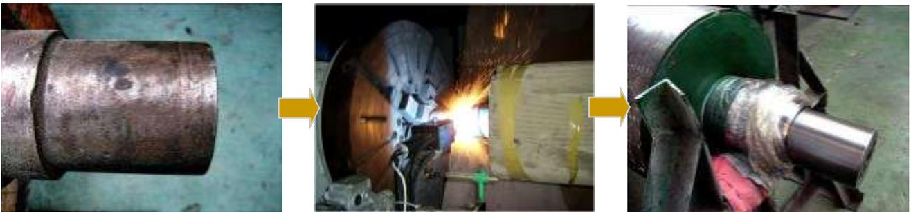
Low temperature Welding technology using pre molten arc that is sprayed into the surface of the work piece.
